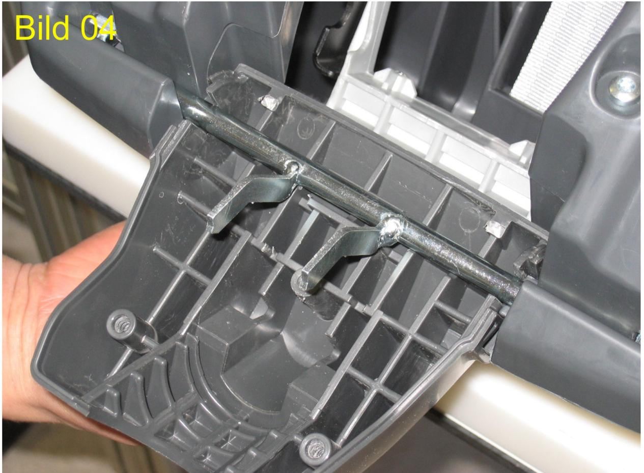
5. Put the positioned support leg in and pay attention to the correct position (!); photo 05 and 06
