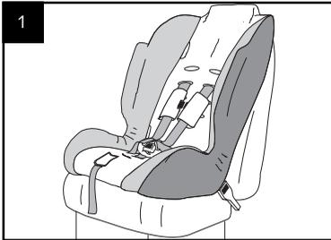
1. Where possible, remove the vehicle seat head-rest. Then place the Traveller Plus on the vehicle seat. Fasten the buckle and pull the harness taut.
