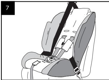
7. The Traveller Plus should now be secure. To check this, try to pull the seat forward by the harness. It should feel firm, not loose.
