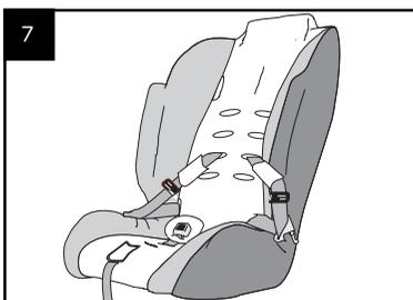
7. Unfasten the chest clip and loosen the harness. Then unfasten the buckle by pressing the red button
