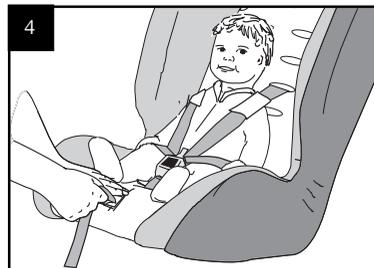
4. Pull the adjuster strap forward making sure the harness is a comfortable but FIRM fit around your child.
