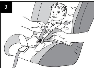
3. Make sure the harness is not twisted and gently pull it up to tighten the lap sections. Make sure the lap straps are kept low down on your child's body by, if necessary, shortening the length of the crotch strap - see *Changing the length of the crotch strap* on page 7.
