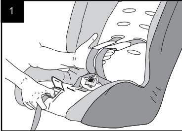
1. With one hand, press and hold down the harness adjuster tab. Then, with the other hand below the chest pads, pull the shoulder straps forwards.
