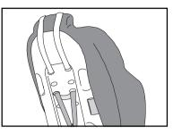
Head Support If the head support is being used, always make sure that its straps are routed through the top shoulder slots and over the top of the Traveller Plus.
