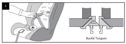
3. Re-thread the straps through the side slots of the cover and shell so that the metal tabs are now back in their original position under the seat. Re-secure them using the cover elastic. Pull the harness straps forward to remove any slack. Make sure the harness straps are not twisted and are threaded through the buckle tongues as shown.
